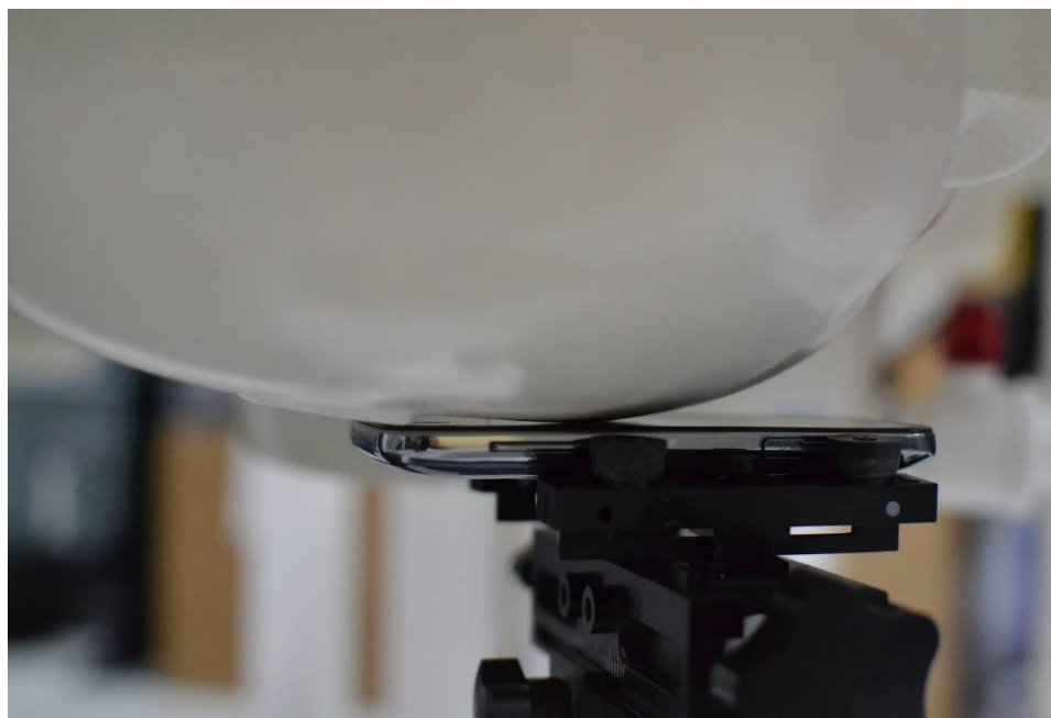
SAR Test Setup Photo 1 – Right Cheek
