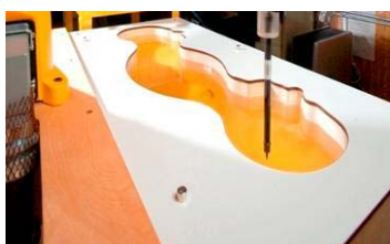
Figure 6-2 SAM Phantom with Simulating Tissue
