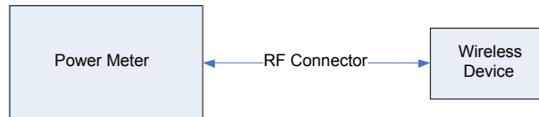
Figure 10-1 Power Measurement Setup
