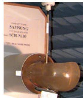
Fig. 1 SAR Test Setup
