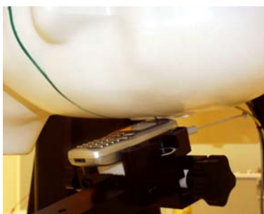
Figure 8.5 Left Head SAR Test Setup -- Ear/Tilt 15° Position--
