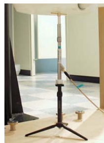
Figure 7.1 Dipole Validation Test Setup
