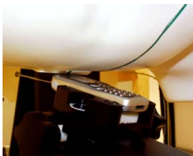
Figure 8.3 Right Head SAR Test Setup -- Ear/Tilt 15° Position--
