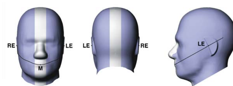
Figure 5.1 Front, back and side view of SAM
