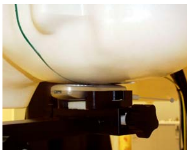
Figure 8.4 Left Head SAR Test Setup -- Cheek / Touch Position--
