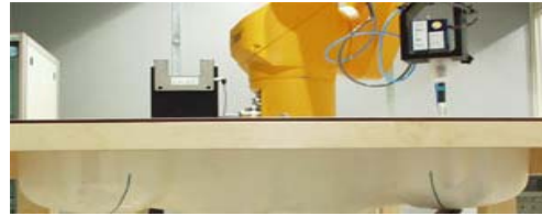
Figure 3.5 SAM Twin Phantom
