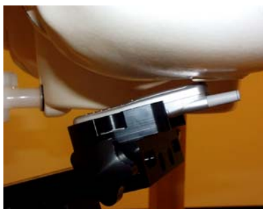
Figure 8.5 Left Head SAR Test Setup -- Ear/Tilt 15° Position--
