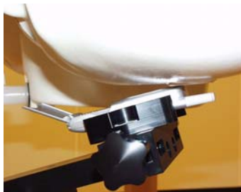
Figure 8.10 Left Head SAR Test Setup -- Ear/Tilt 15° Position--
