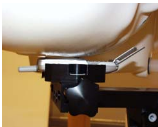
Figure 8.2 Right Head SAR Test Setup --Cheek/Touch Position--
