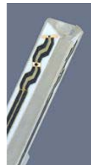
Figure 3.4 Probe Thick-Film Technique
