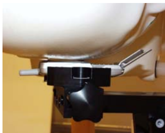
Figure 8.7 Right Head SAR Test Setup -- Cheek / Touch Position--
