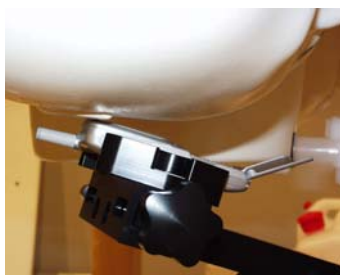
Figure 8.8 Right Head SAR Test Setup -- Ear/Tilt 15° Position--
