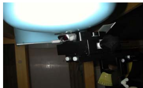
Figure 19. Right Head SAR Test Setup -- Ear / Tilt Position --
