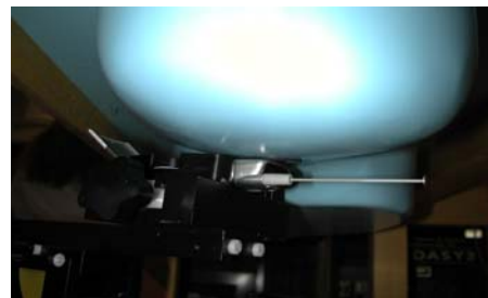
Figure 17. Left Head SAR Test Setup -- Ear / Tilt Position --
