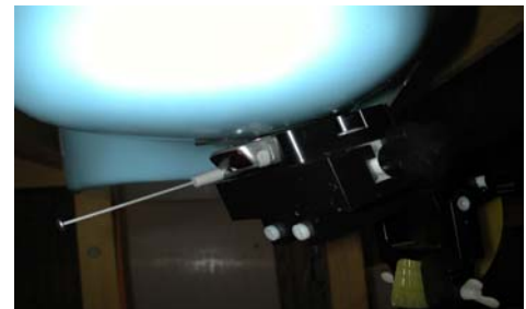
Figure 18. Right Head SAR Test Setup -- Check / Touch Position --
