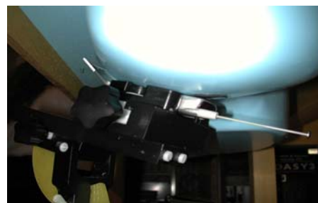
Figure 16. Left Head SAR Test Setup -- Check / Touch Position --
