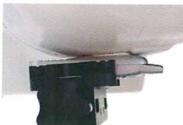
Figure 8.8 Left Head SAR Test Setup -- Cheek / Touch Position--
