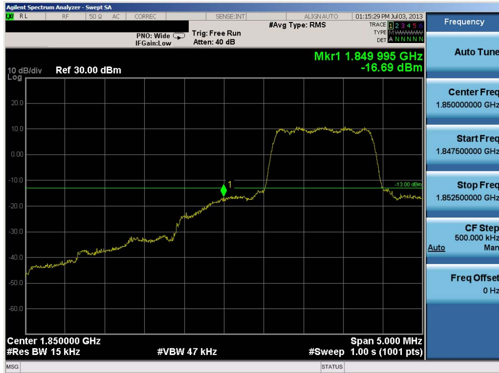
Plot 6-29. Band Edge Plot (PCS CDMA Mode – Ch. 25)
