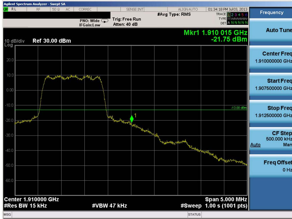
Plot 6-31. Band Edge Plot (PCS CDMA Mode – Ch. 1175)
