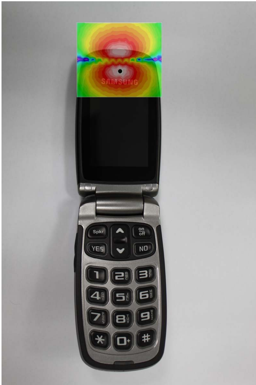
Scan Overlay with actual device (Radial Longitudinal)
