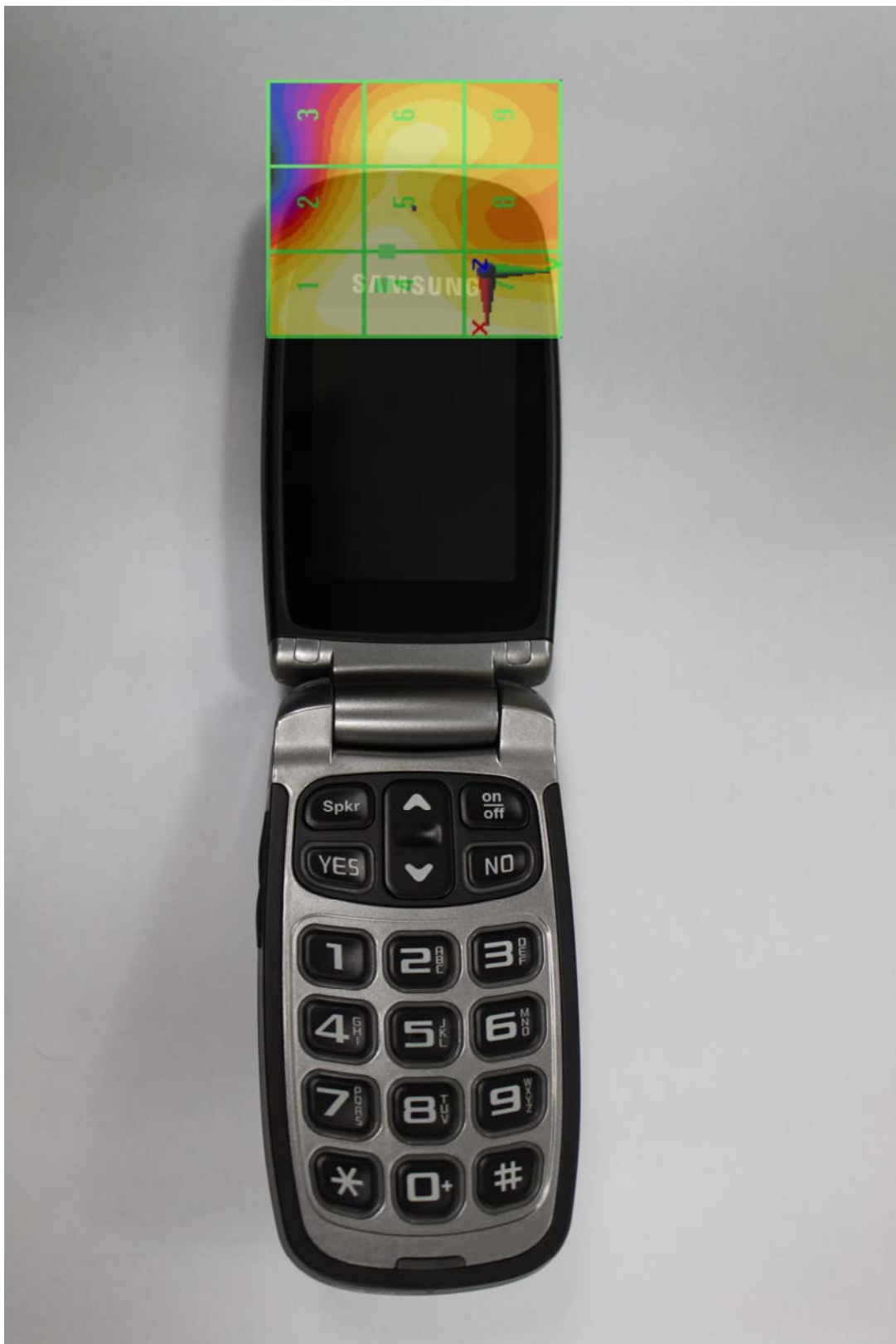
Scan Overlay with actual device(E-Field)
