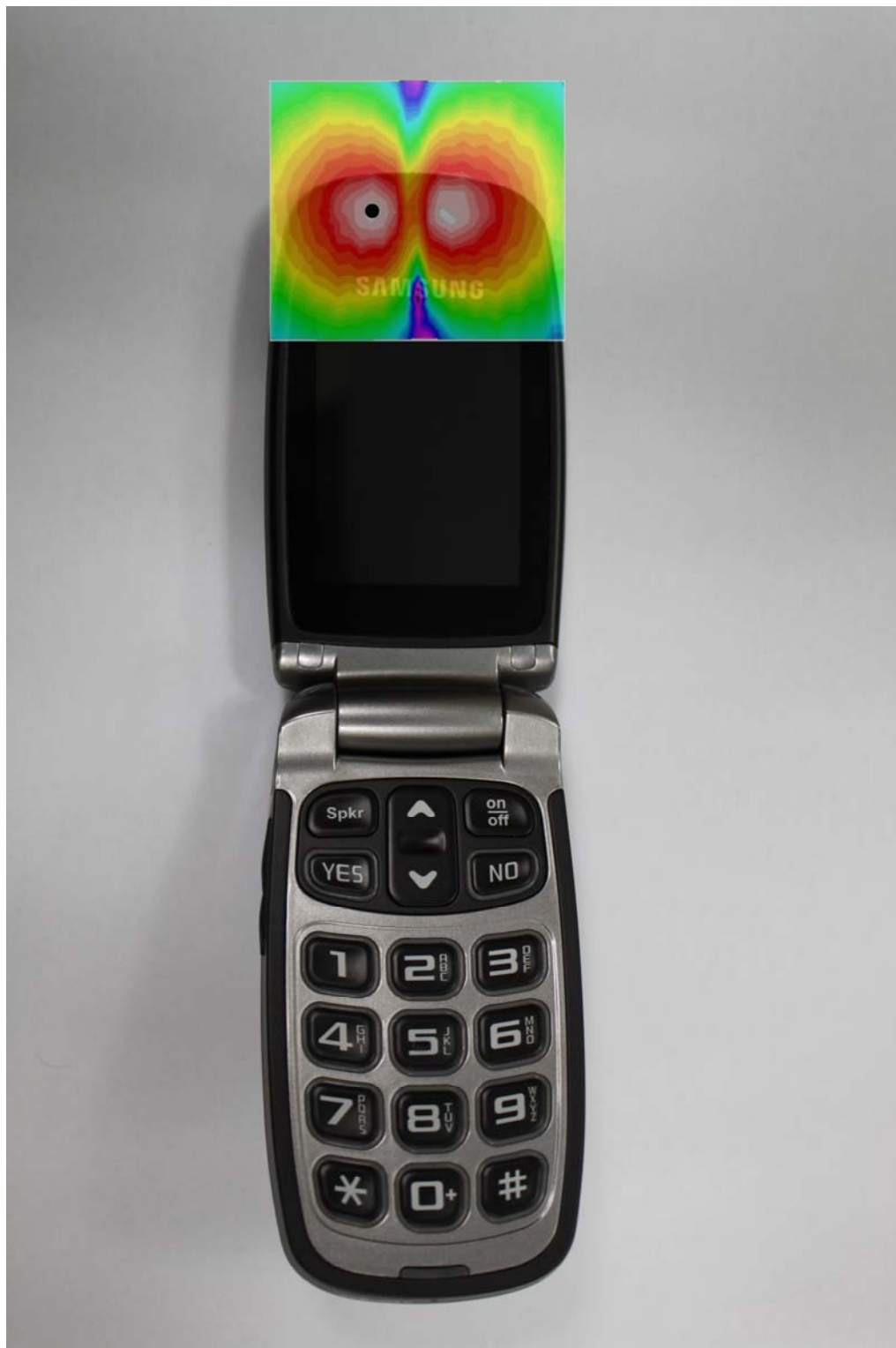
Scan Overlay with actual device (Radial Transverse)
