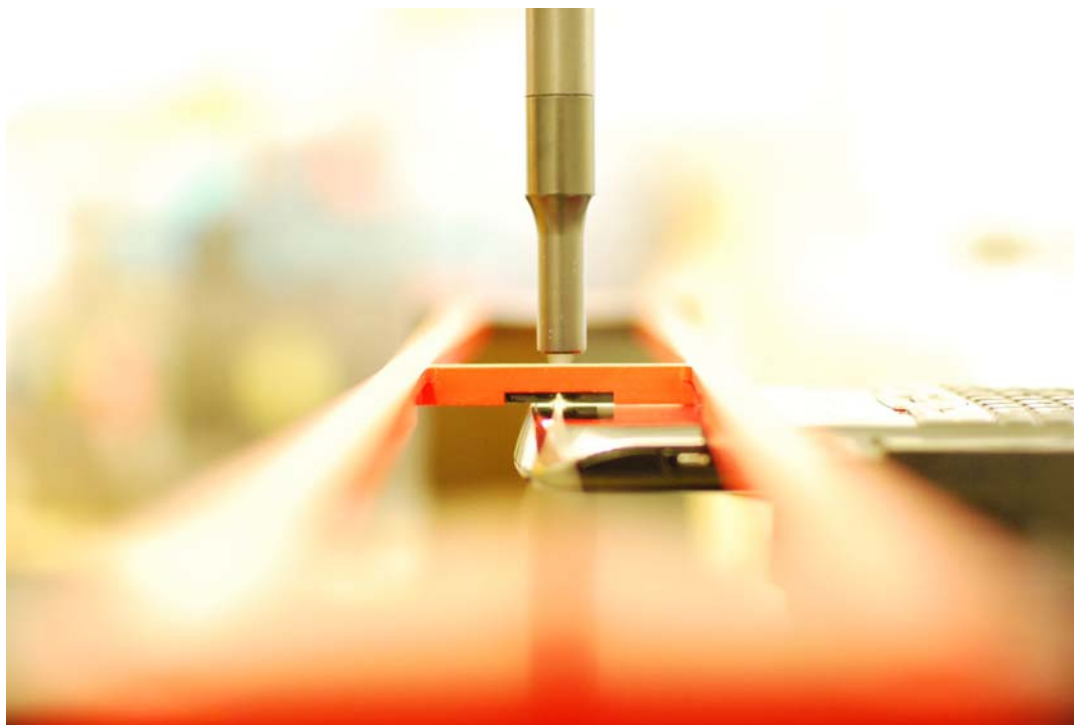
Figure 17-2 HAC Phantom Plane Alignment
