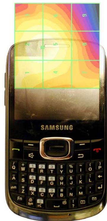
Figure 17-5 H-Field WD Scan overlay
