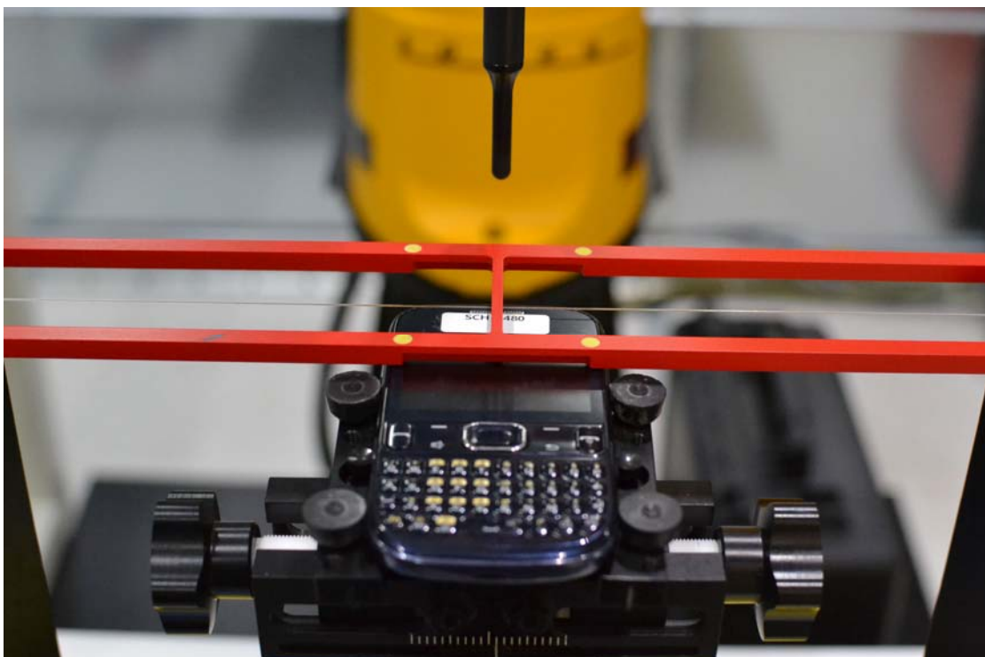
Figure 17-1 Ear Reference Point HAC Phantom Alignment
