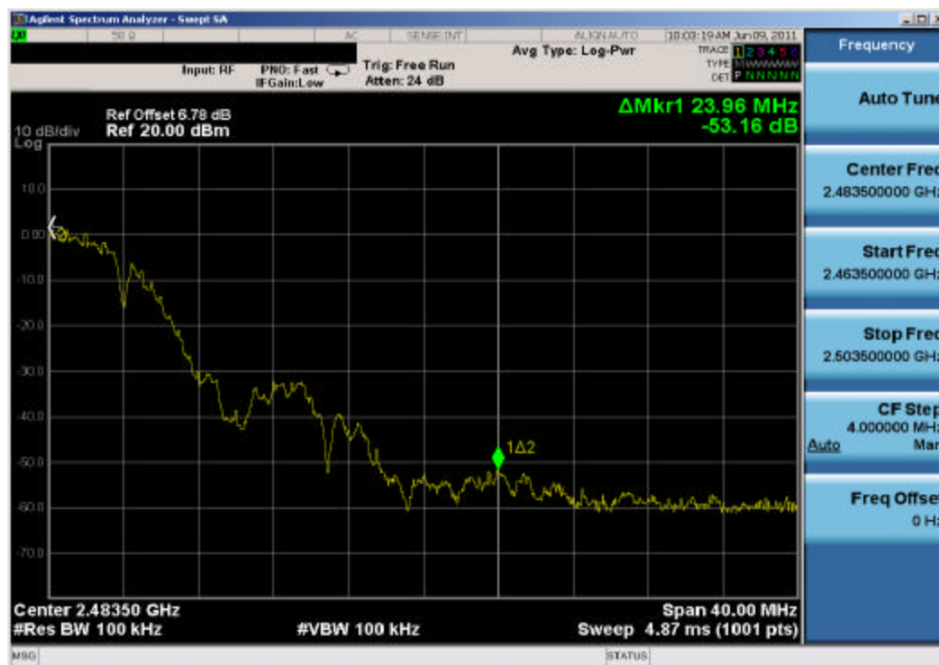
Plot 6-20. Band Edge Plot (802.11b – Ch. 11)
