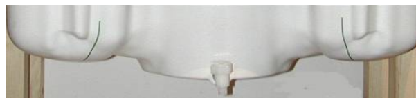
Figure 7-2 SAM Twin Phantom Shell
