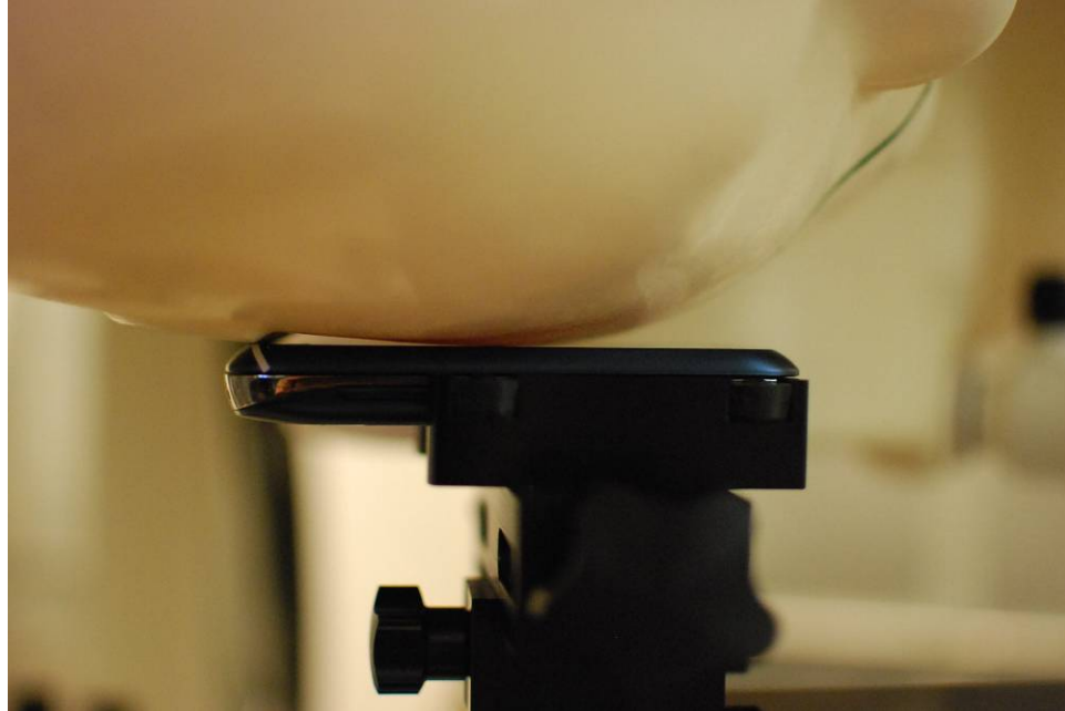
SAR Test Setup Photo 1: Right Touch
