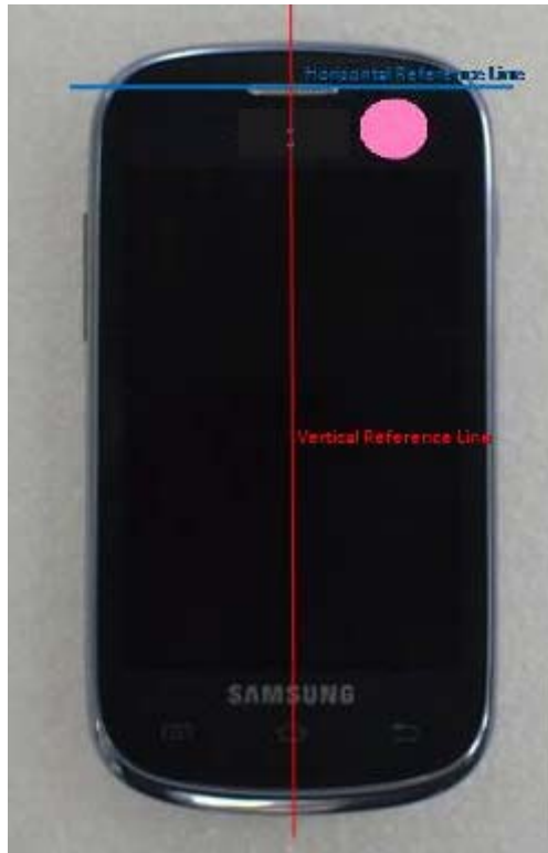
SAR Test Setup Photo 11 – Vertical and Horizontal Reference Lines
