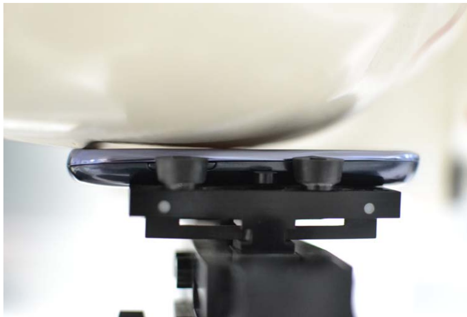
SAR Test Setup Photo 1 – Right Cheek
