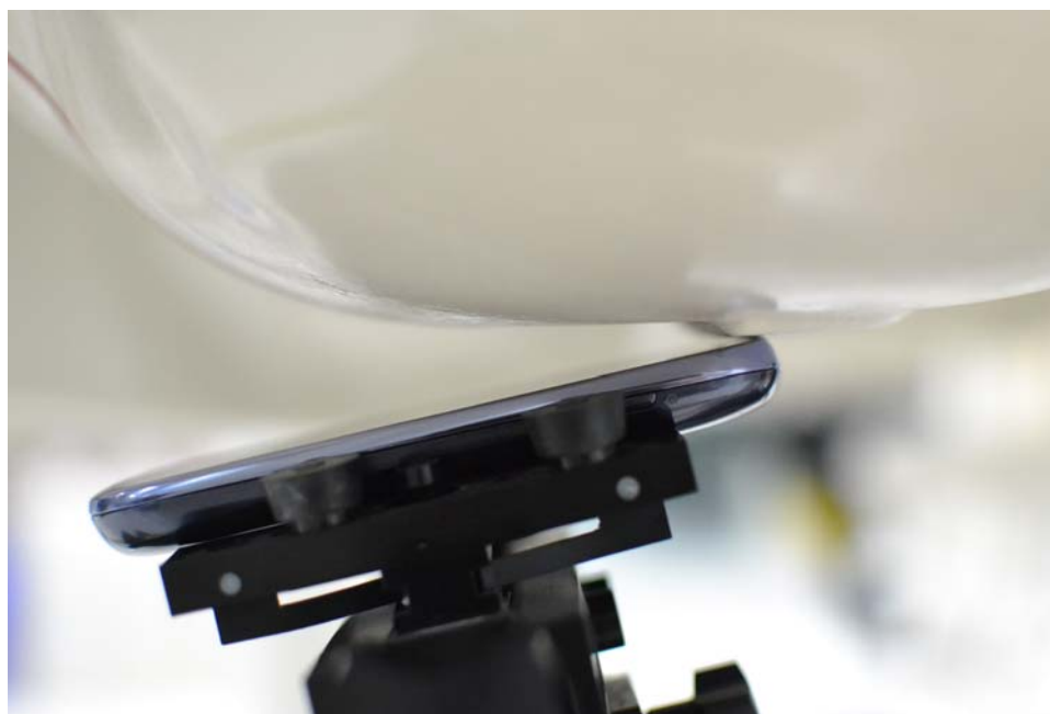
SAR Test Setup Photo 4 – Left Tilt
