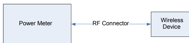
Figure 13-9 Power Measurement Setup
