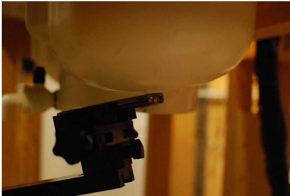
SAR Test Setup Photo 4: Left Tilt
