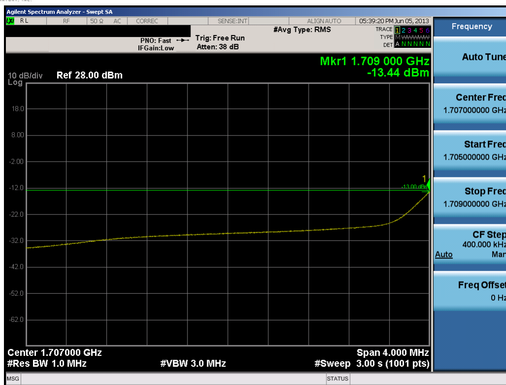
Plot 10-2. Lower Extended Band Edge Plot (5.0MHz QPSK – RB Size 25)
