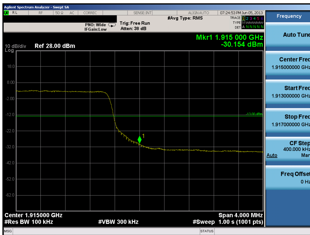
Plot 12-25. Upper Band Edge Plot (10.0MHz QPSK – RB Size 50)
