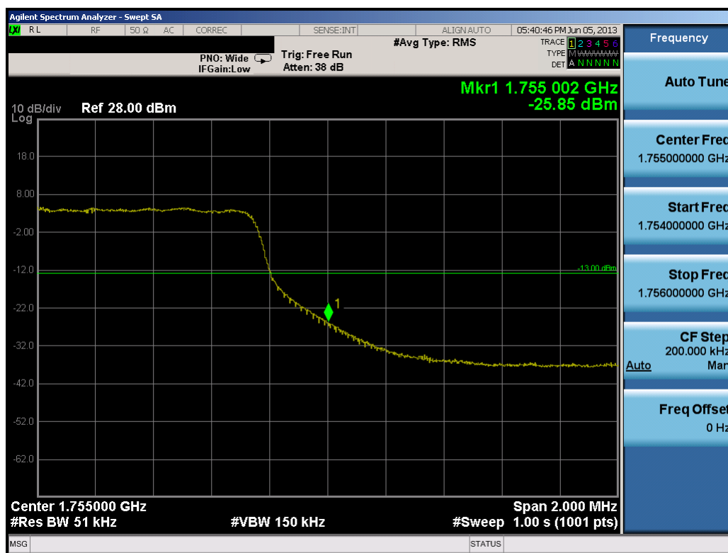
Plot 10-11. Upper Band Edge Plot (5.0MHz QPSK – RB Size 25)
