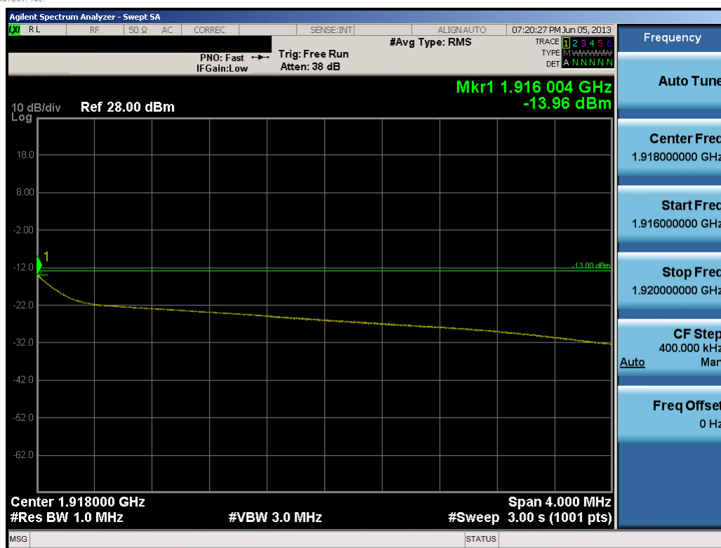
Plot 12-12. Upper Extended Band Edge Plot (5.0MHz QPSK – RB Size 25)
