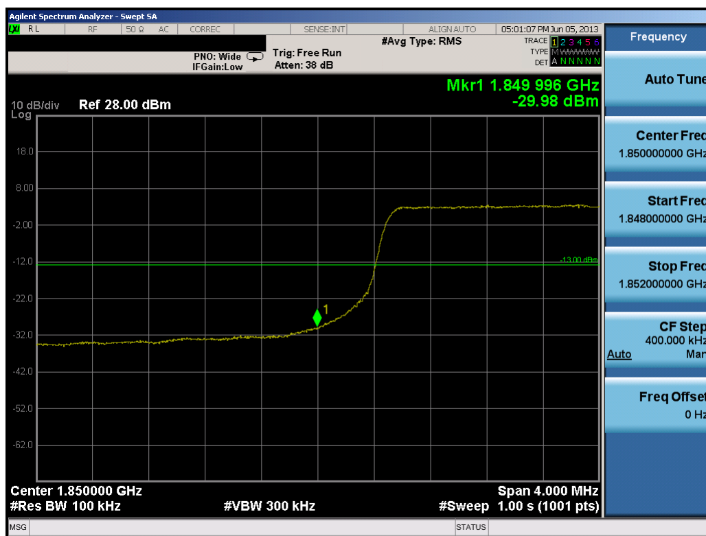
Plot 11-15. Lower Band Edge Plot (10.0MHz QPSK – RB Size 50)
