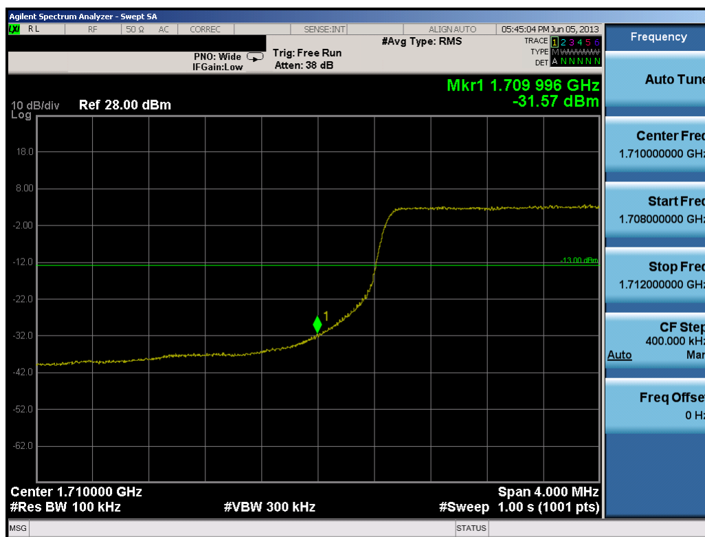
Plot 10-15. Lower Band Edge Plot (10.0MHz QPSK – RB Size 50)
