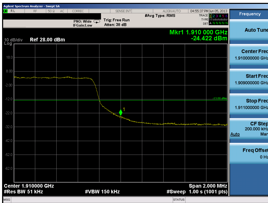
Plot 11-11. Upper Band Edge Plot (5.0MHz QPSK – RB Size 25)
