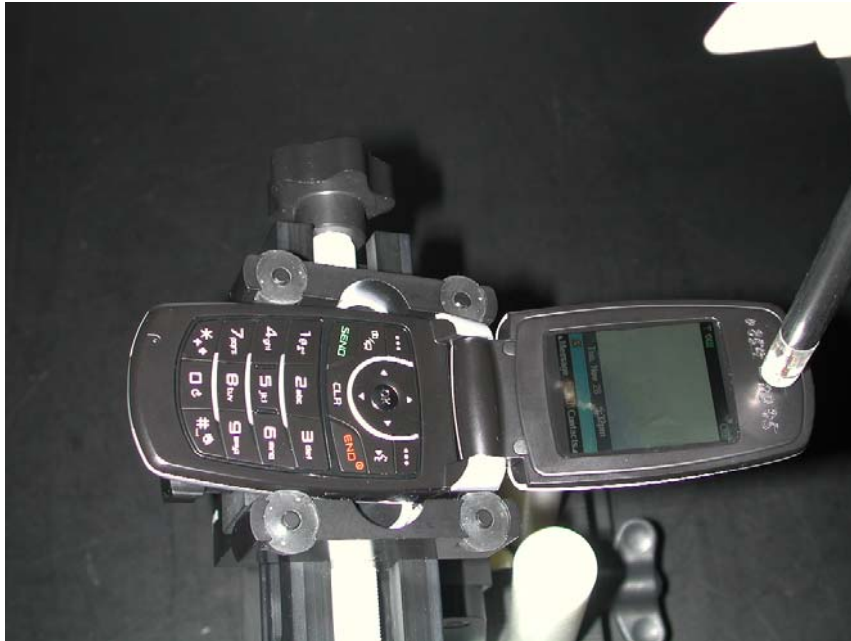
Figure 0-1 Test Setup for Wireless Device
