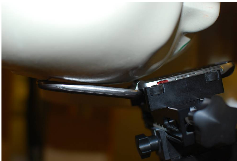
Figure 19-2 SAR Test Setup Photo 2 – Right Touch
