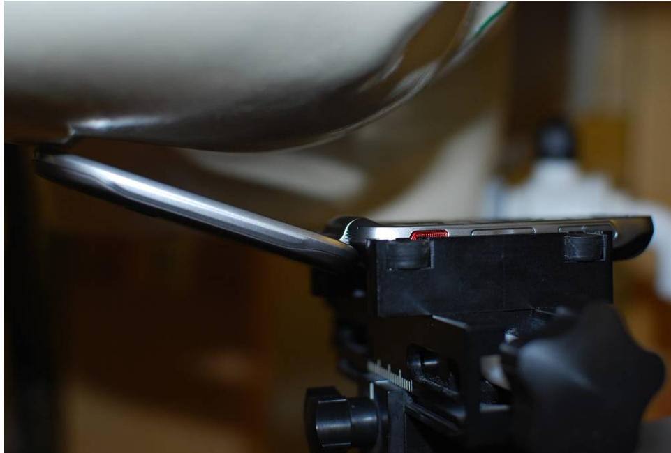
Figure 19-3 SAR Test Setup Photo 3 – Right Tilt
