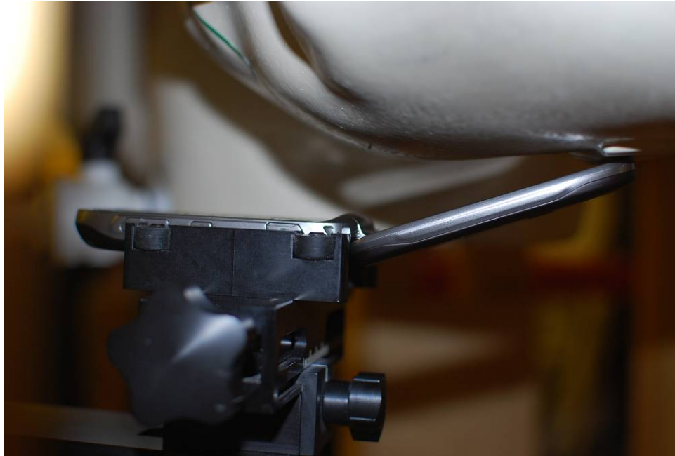
Figure 19-5 SAR Test Setup Photo 5 - Left Tilt
