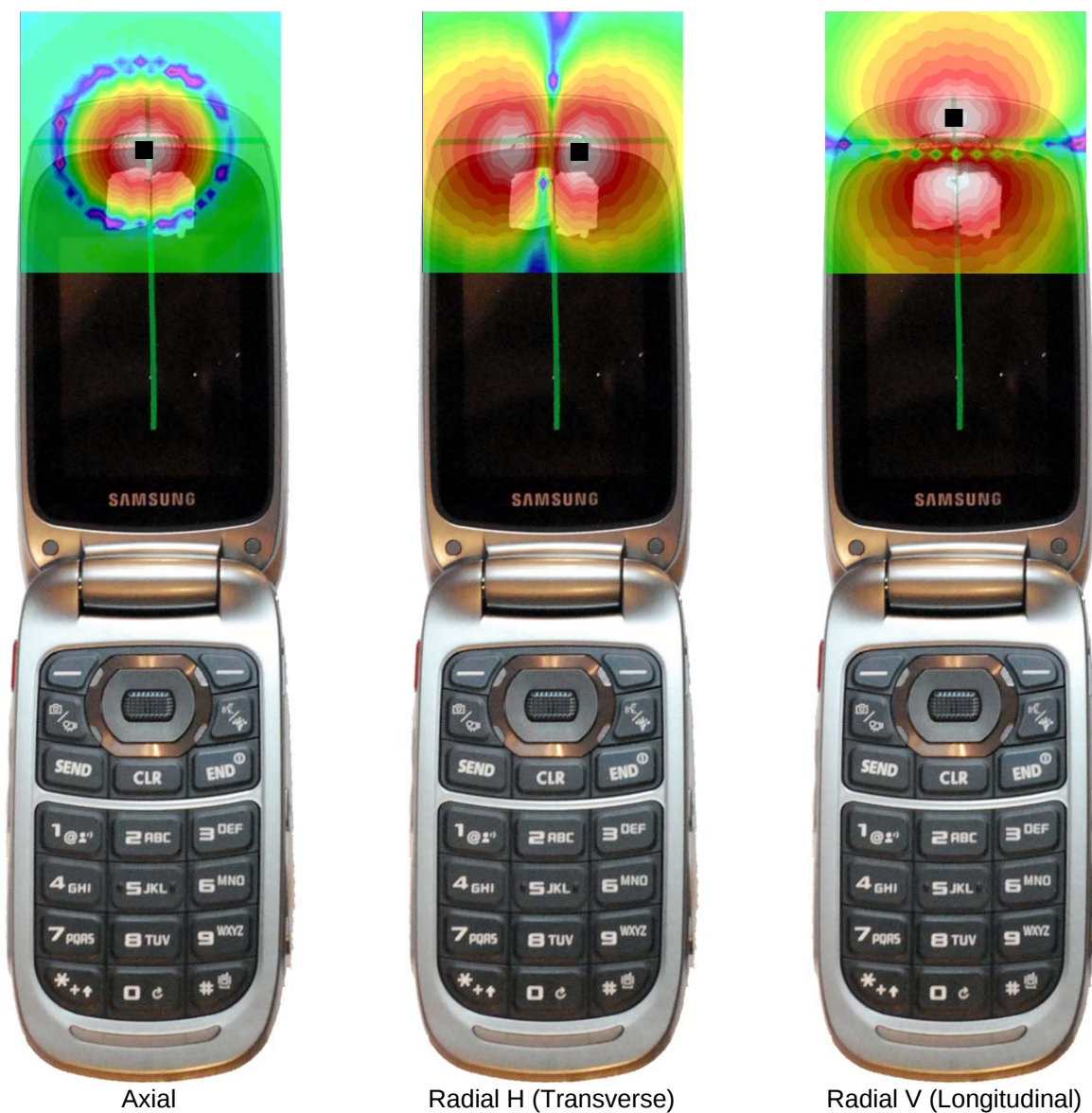
Figure 13-3 T-Coil Scan Overlay Magnetic Field Distributions
