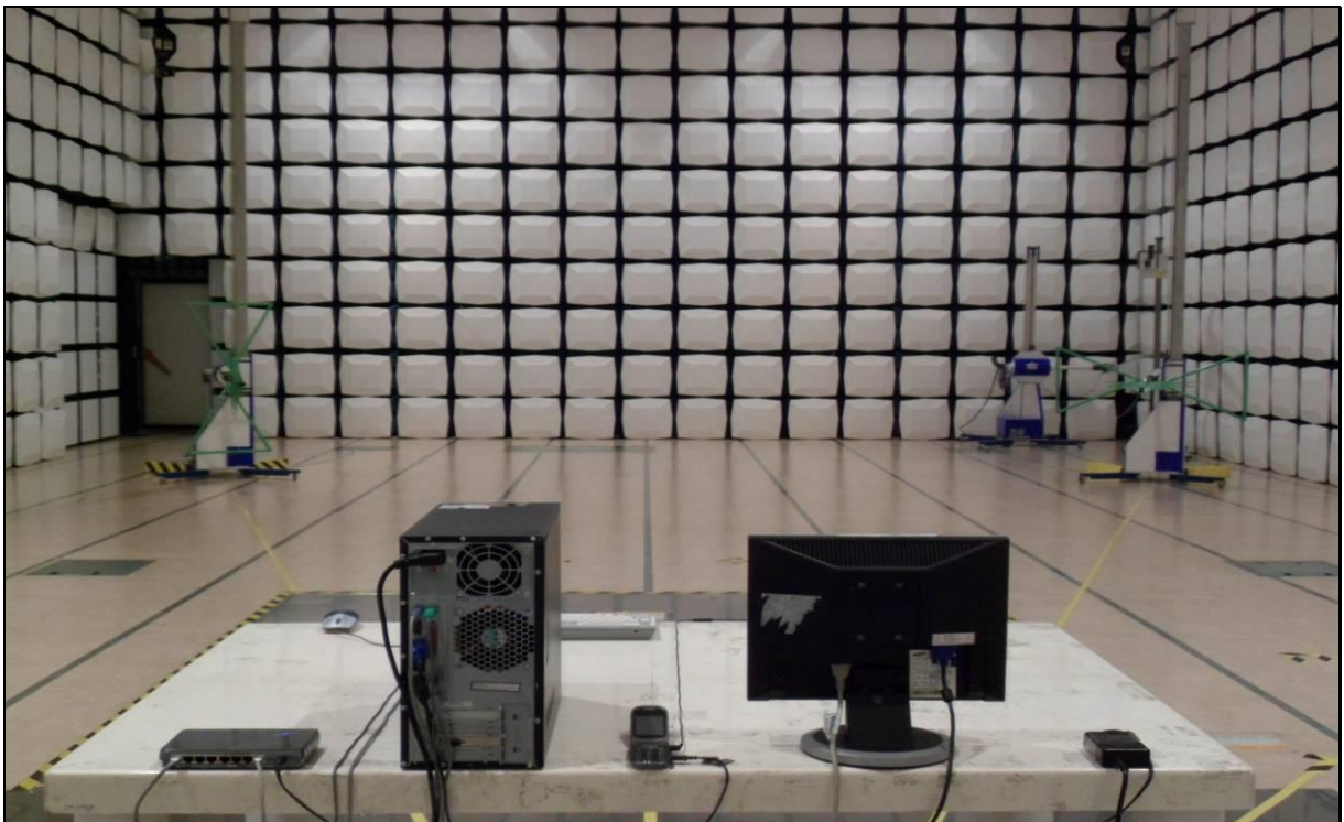
[ Radiated Disturbance for Below 1 GHz – Rear ]
