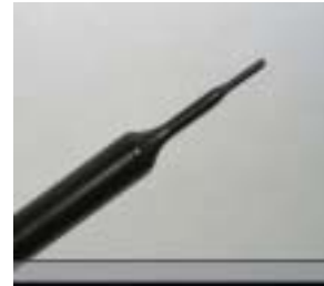
Figure 3.4 Probe Thick-Film Technique
