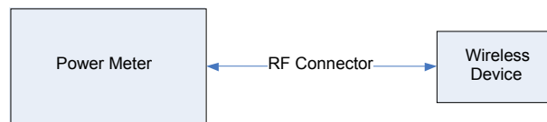
Figure 12-1 Power Measurement Setup
