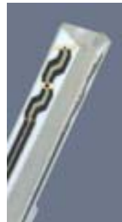
Figure 3.4 Probe Thick-Film Technique
