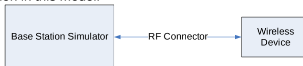
Figure 9-2 Power Measurement Setup
