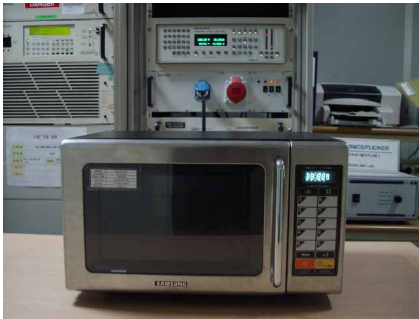
Fig. 2 Test Setup for Input power
