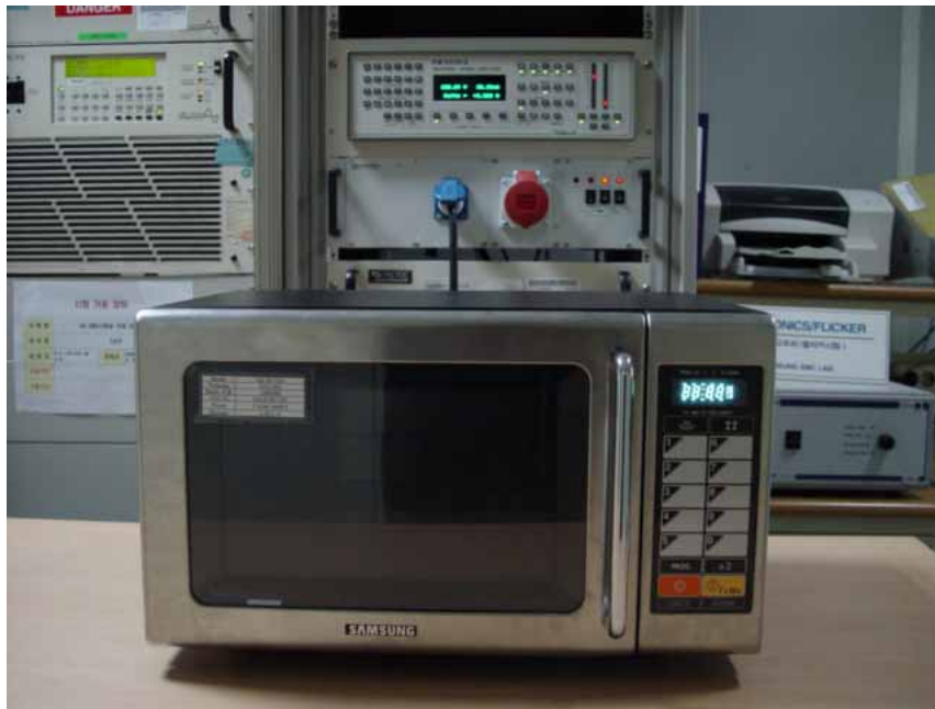
Fig.3 Test Setup for RF output power
