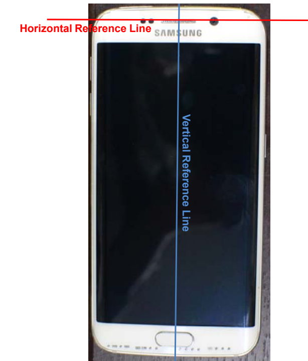
SAR Test Setup Photo 11: Horizontal and Vertical Reference Lines
