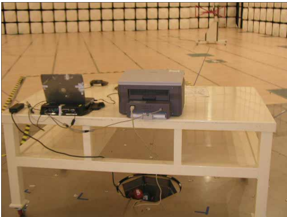
Pic. 4. Radiated Emission (Rear)
