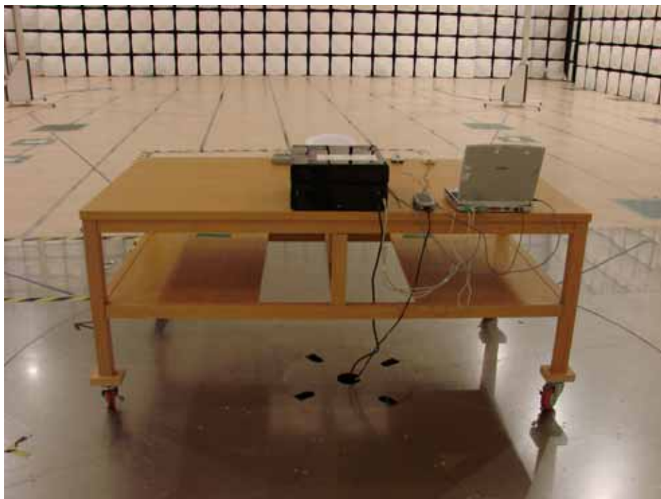
Picture 4. Radiated emission (Rear)
