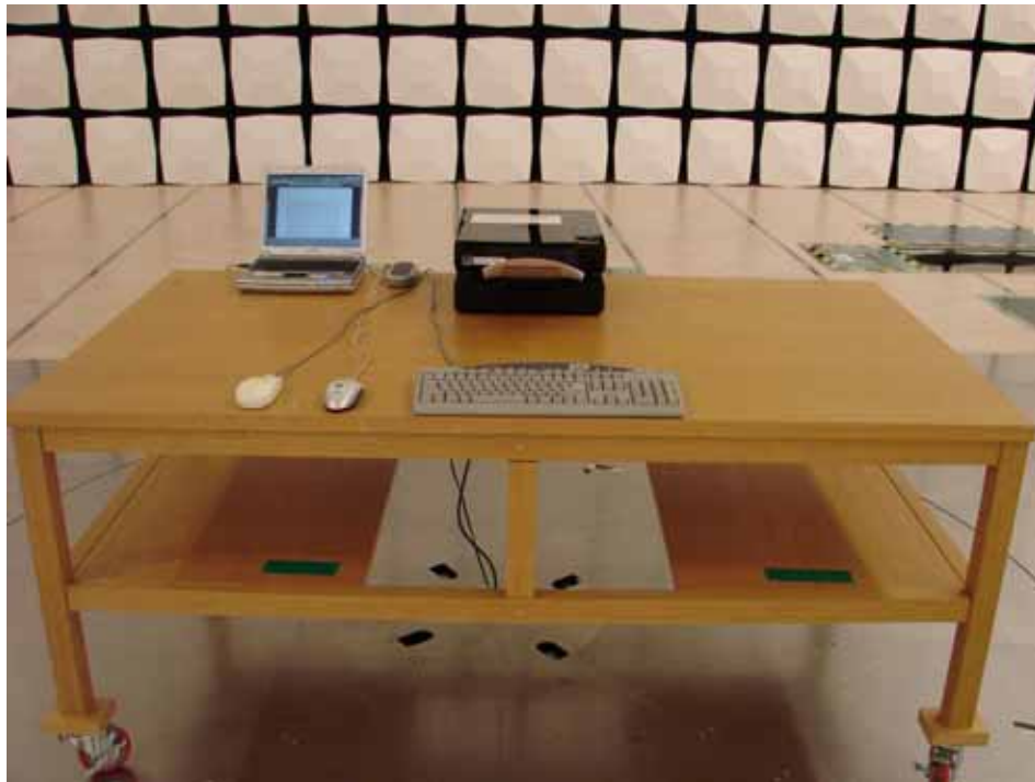
Picture 3. Radiated emission (Front)
