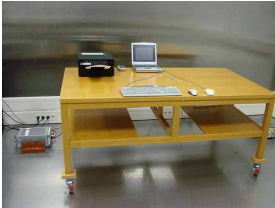
Picture 1. Conducted Emission (Front)
