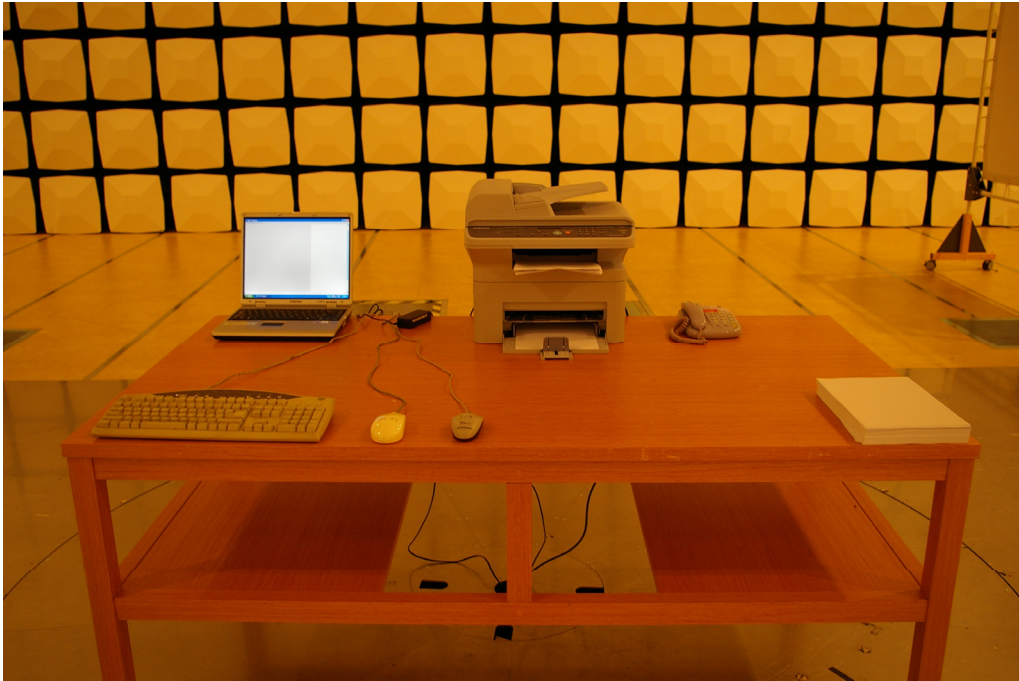
Picture 3. Radiated emission (Front)
