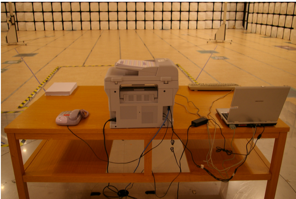
Picture 4. Radiated emission (Rear)
