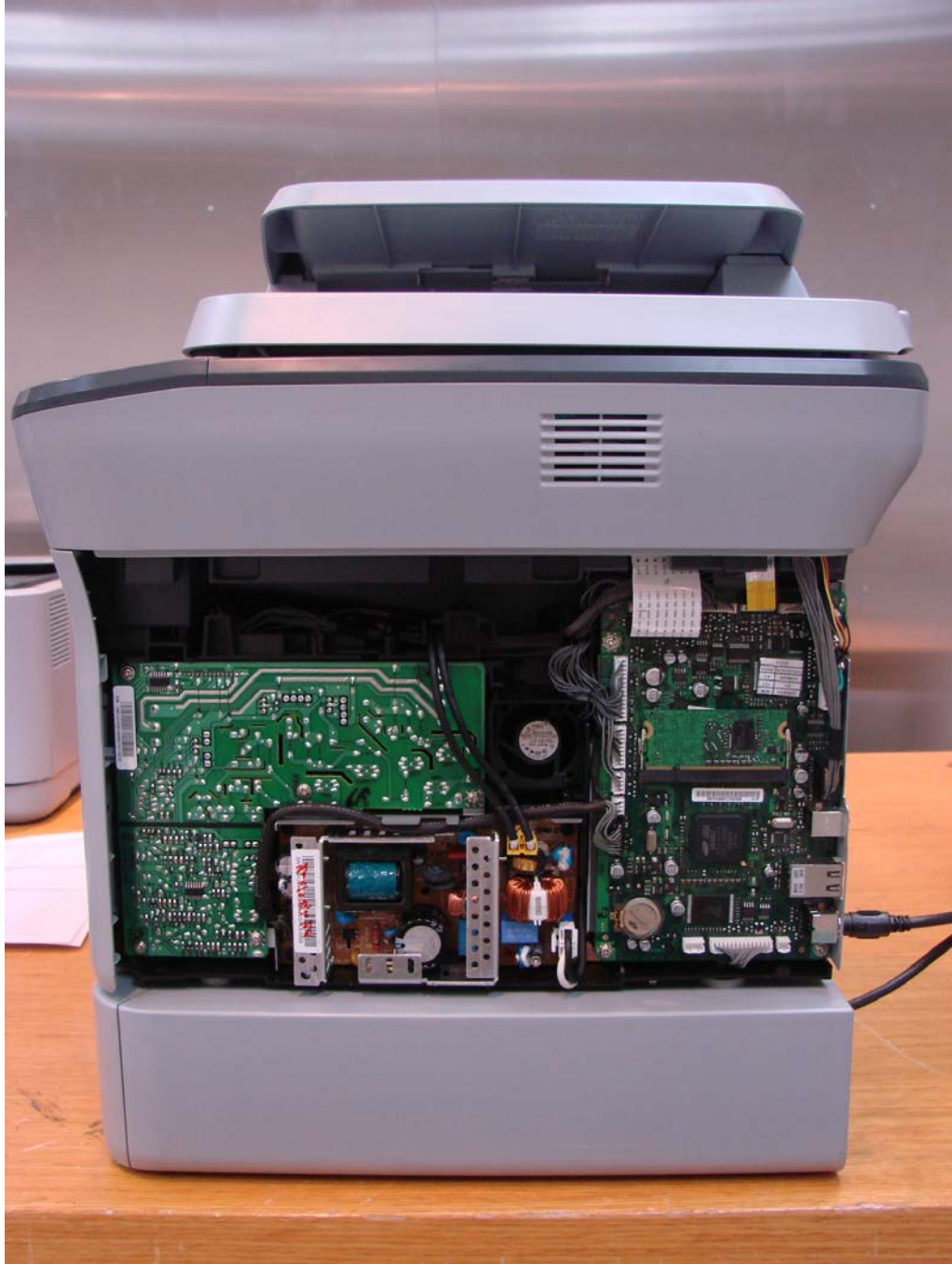
Internal View 2 (Sungho Electronics SMP board)
