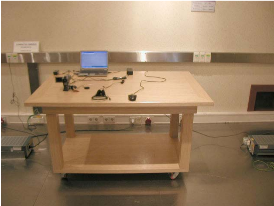
Picture 1. Conducted Emission (Front)
