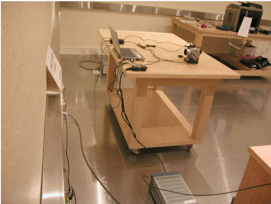
Picture 2. Conducted Emission (Rear)
