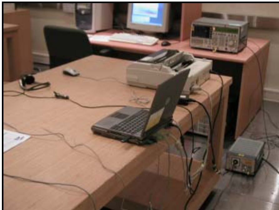
Pic. 2 Conducted Emission (Rear)
