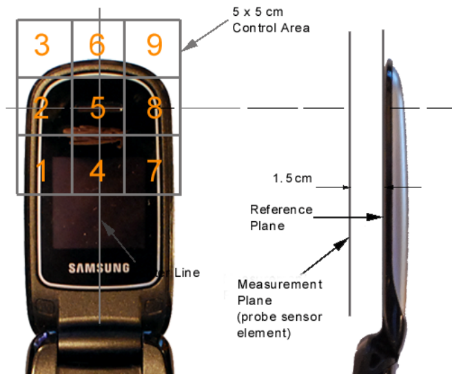
Figure 16-3 5x5 Scan grid above WD
