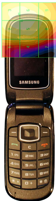
Figure 16-4 E-Field WD Scan overlay
