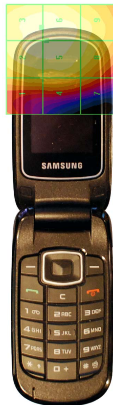
Figure 16-5 H-Field WD Scan overlay
