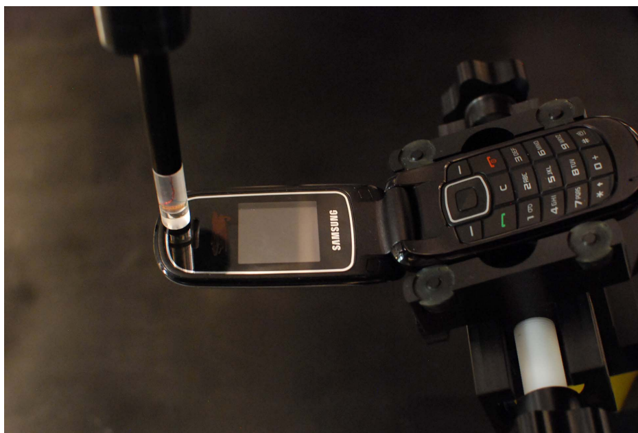
Figure 12-2 Test Setup for Wireless Device
