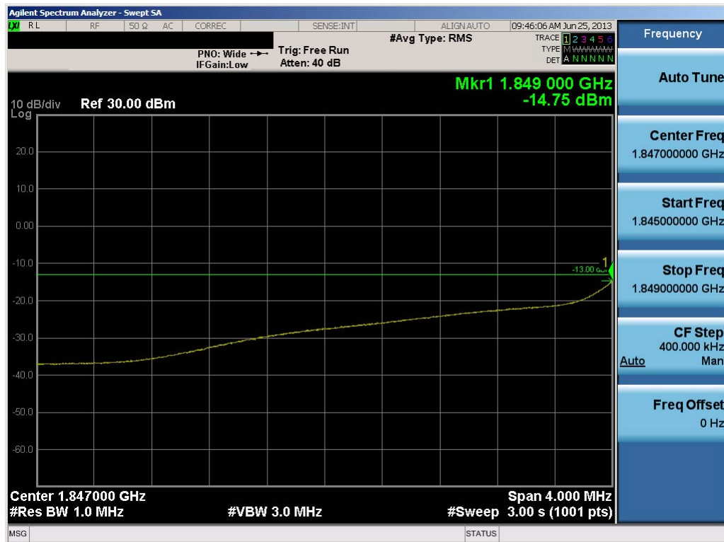
Plot 7-38. 4MHz Span Plot (PCS WCDMA Mode – Ch. 9262)
