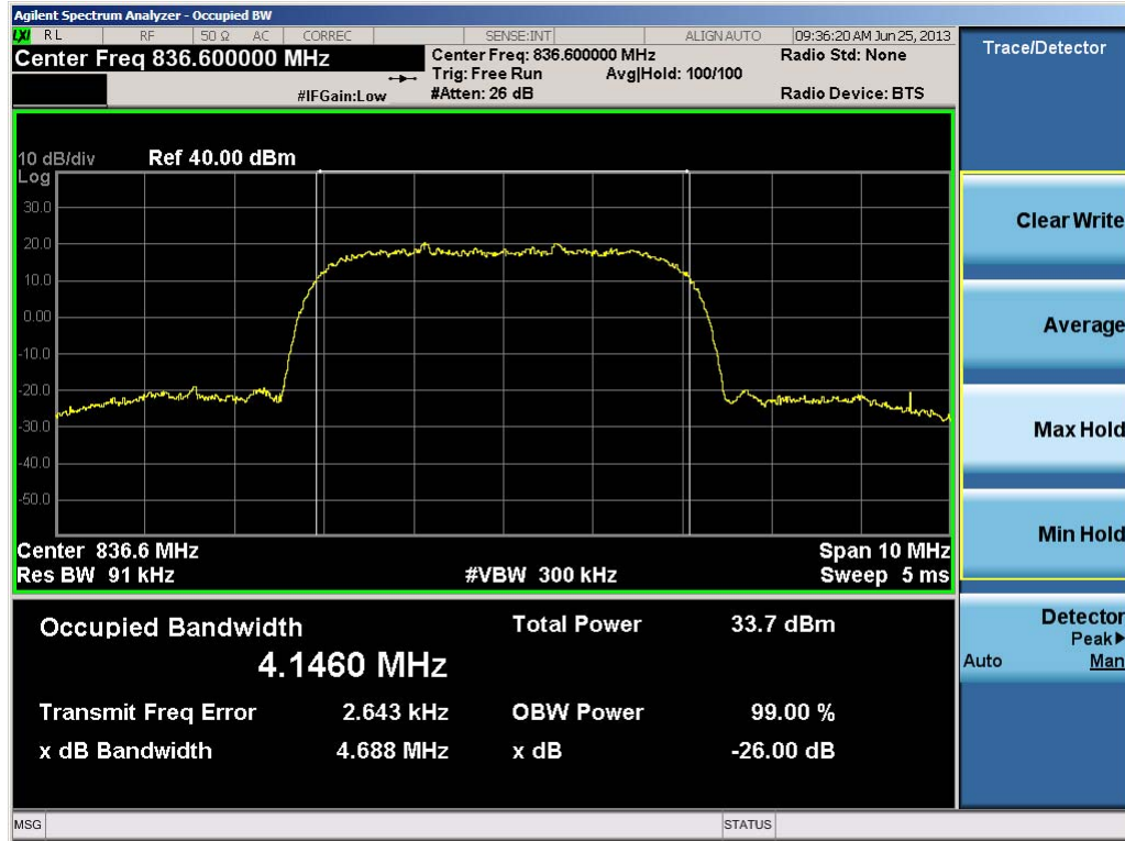
Plot 7-31. Occupied Bandwidth Plot (Cellular WCDMA Mode – Ch. 4183)
