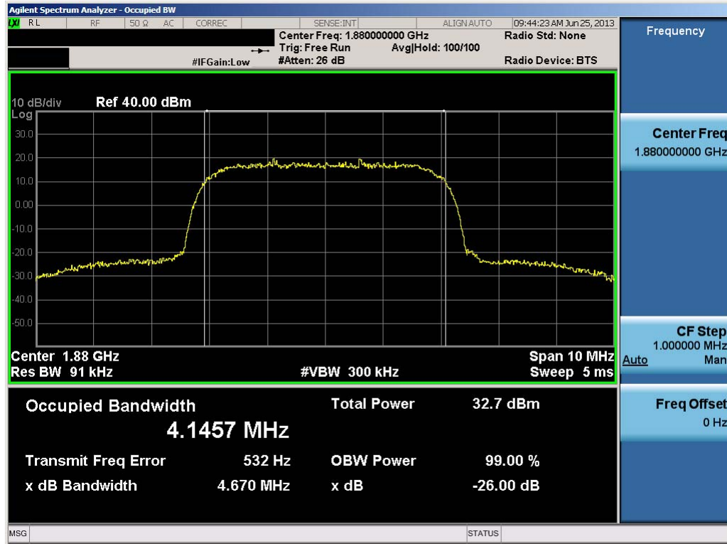
Plot 7-41. Occupied Bandwidth Plot (PCS WCDMA Mode – Ch. 9400)
