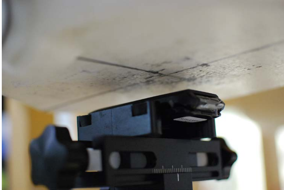
SAR Test Setup Photo 8: Body-worn at 1.5 cm
