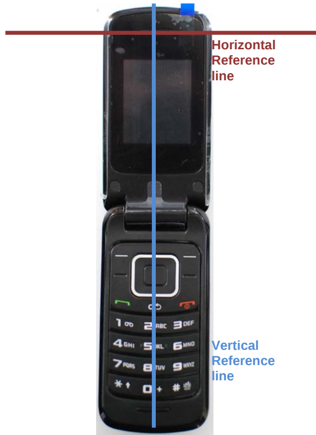
SAR Test Setup Photo 8: DUT Reference Lines
