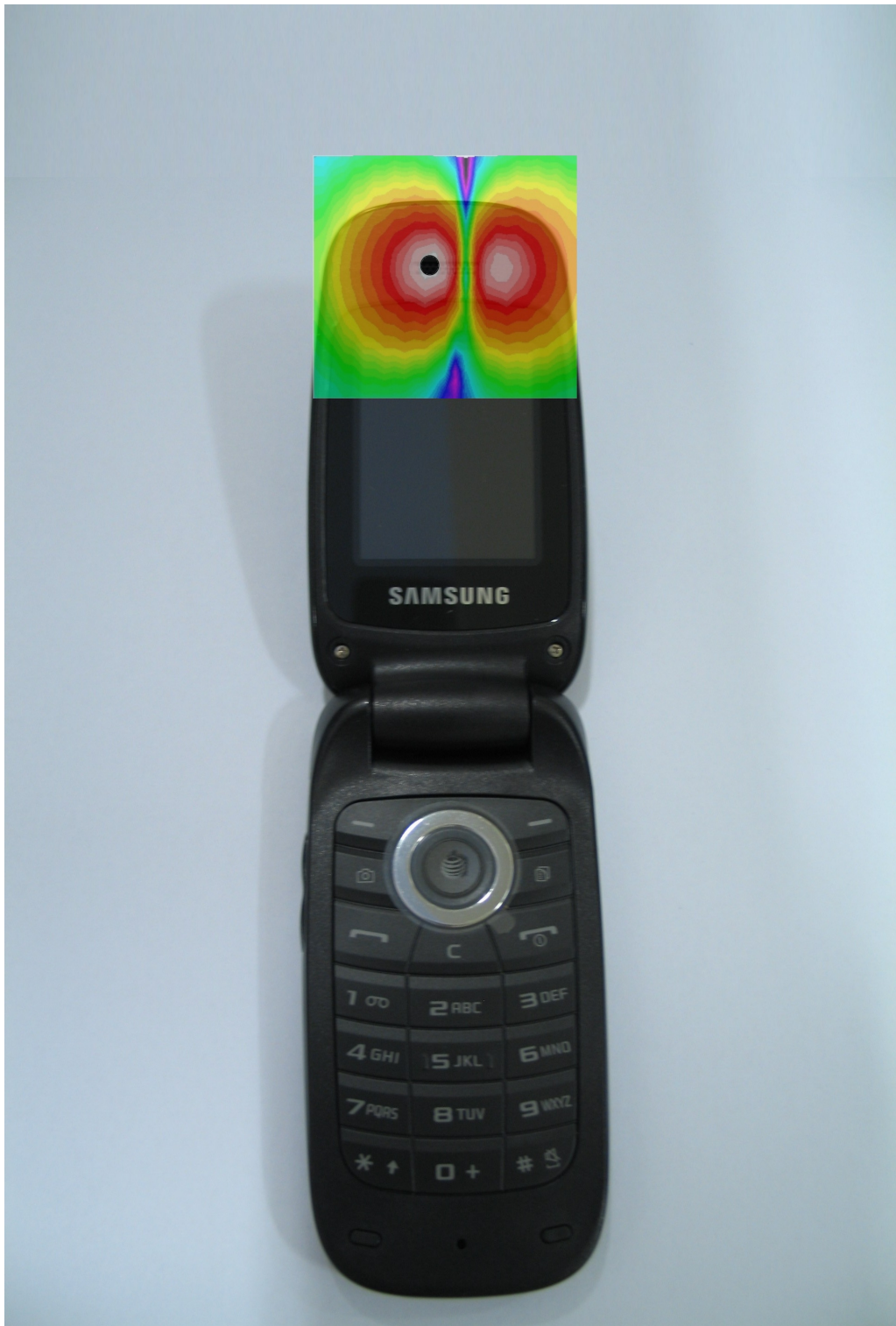
Scan overlay with actual device (Radial Transverse)
