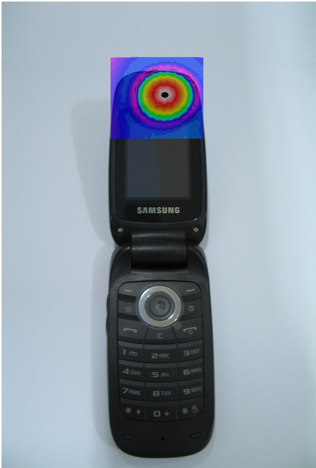
Scan overlay with actual device (Axial)
