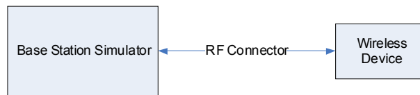
Figure 12-1 Power Measurement Setup
