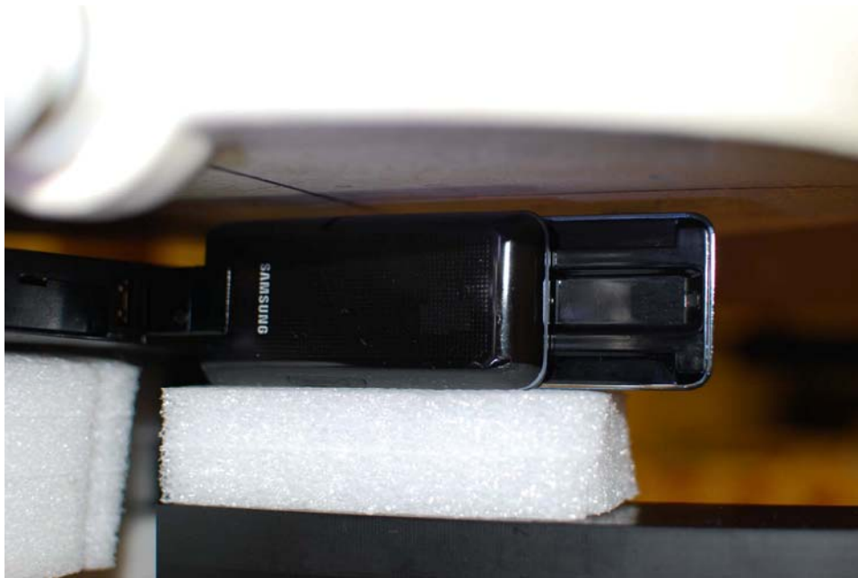
Figure 17-4 SAR Test Setup: Left
