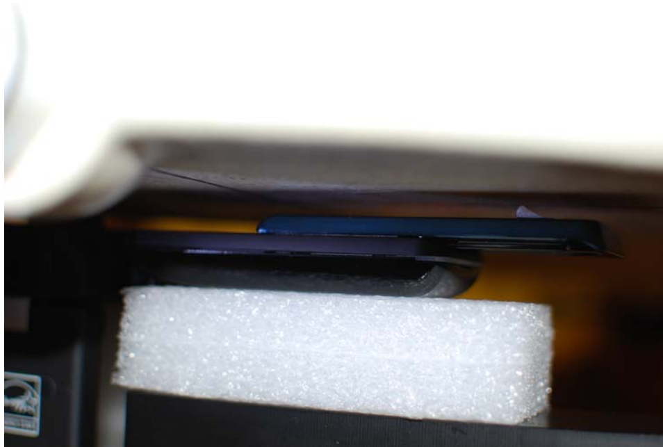
Figure 17-1 SAR Test Setup: Front
