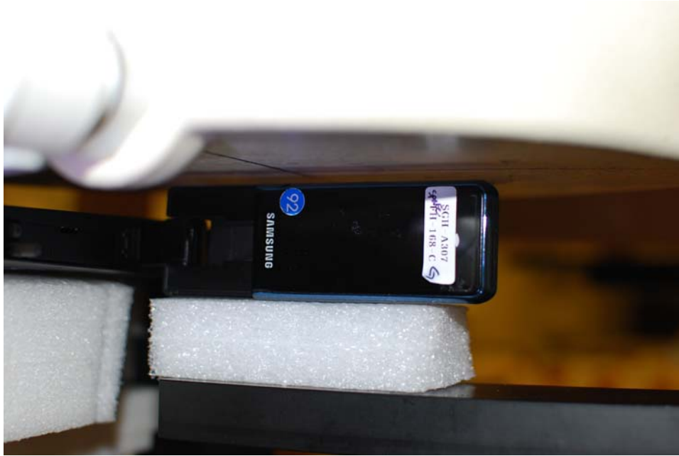
Figure 17-3 SAR Test Setup: Right
