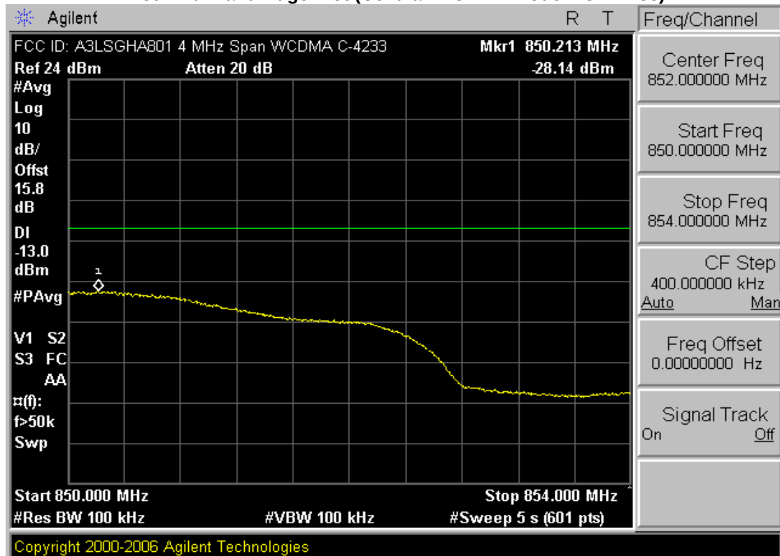
Plot 7-21. 4MHz Span Plot (Cellular WCDMA Mode – Ch. 4233)
