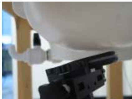
Figure 8.3 Right Head SAR Test Setup -- Ear/Tilt 15° Position--
