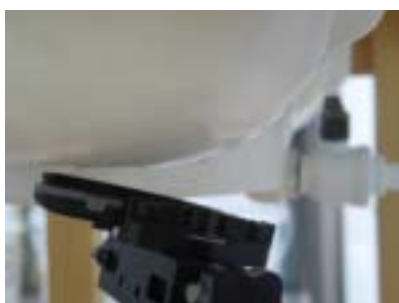
Figure 8.5 Left Head SAR Test Setup -- Ear/Tilt 15° Position--
