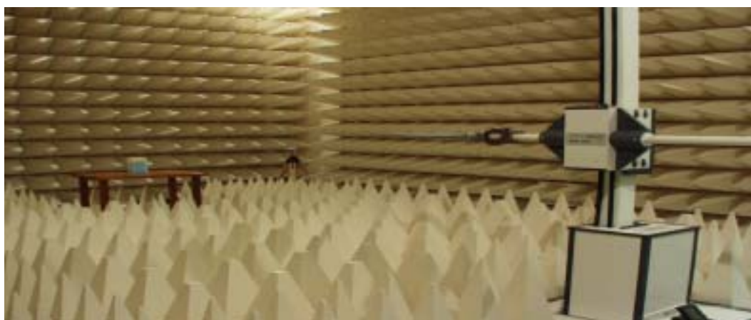
Figure2. Photograph of 3m Fully-Anechoic Chamber
