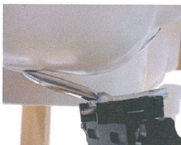
Figure 8.3 Right Head SAR Test Setup -- Ear/Tilt 15° Position--
