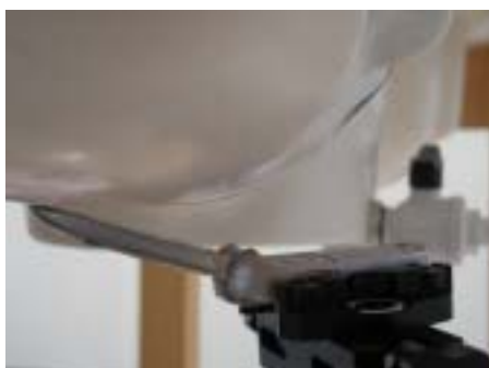
Figure 8.3 Right Head SAR Test Setup -- Ear/Tilt 15° Position--
