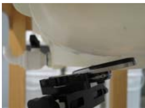
Figure 8.5 Left Head SAR Test Setup -- Ear/Tilt 15° Position--
