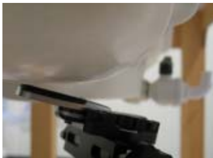
Figure 8.7 Right Head SAR Test Setup -- Ear/Tilt 15° Position--
