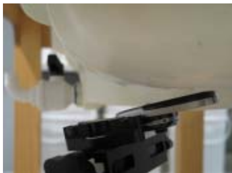
Figure 8.9 Left Head SAR Test Setup -- Ear/Tilt 15° Position--
