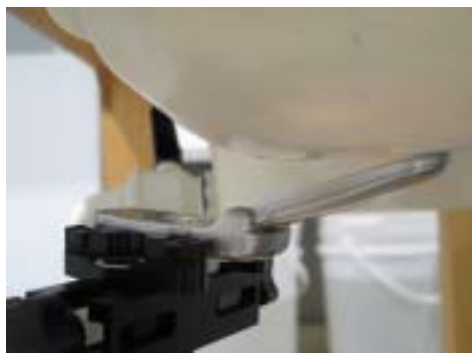
Figure 8.9 Left Head SAR Test Setup -- Ear/Tilt 15° Position--
