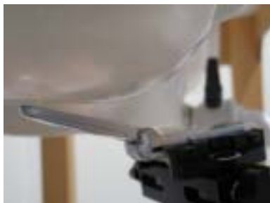
Figure 8.7 Right Head SAR Test Setup -- Ear/Tilt 15° Position--
